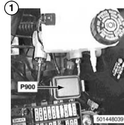
1 P900 AUXILIARY FUSE BOX
